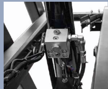
Explosion proof valve, To prevent the machine falling when the oil pipe is leaking
