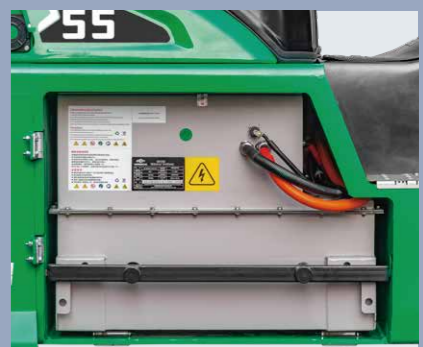
A laterally-removed roller-equipped battery compartment
