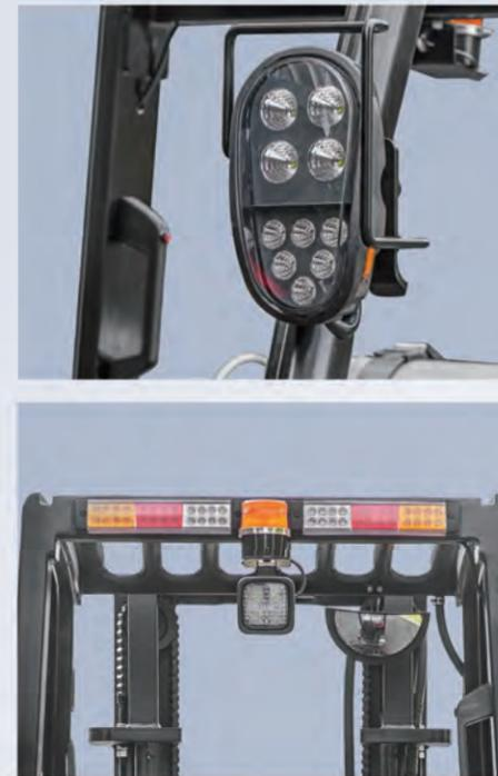
LED lights are used throughout the entire truck. The lights are energy efficient, have a longer service life, and offer a significant increase in performance.
