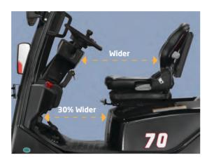
The foot space is now 30% wider to significantly reduce operator fatigue. The new wide, non-slip step makes getting in and out of the forklift safe and easy.
