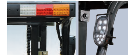
Efficient LED Lighting System
