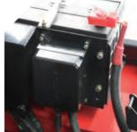
The controllers, relays, and safety fuses are all placed in the dust and water-free controller box. The main electronic components are also waterproof. This allows the operator to use the forklift in wet environments.
