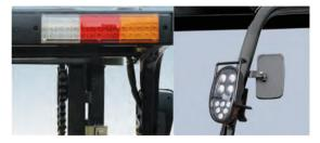
The new efficient lighting system uses LEDs and a new type of reflector to reduce energy consumption. This significantly improves illumination performance while also prolonging operation time.
