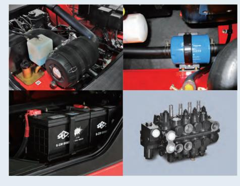
The brake and steering hydraulic systems are separated to prevent interference between each other and increase reliability.
