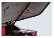
There is a locking mechanism found on the engine hood, damper, and parking brake for the operator's safety.
