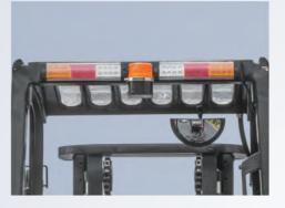
LED lights are used throughout the entire truck. The lights are energy-efficient, have a longer service life, and offer a significant increase in performance.
